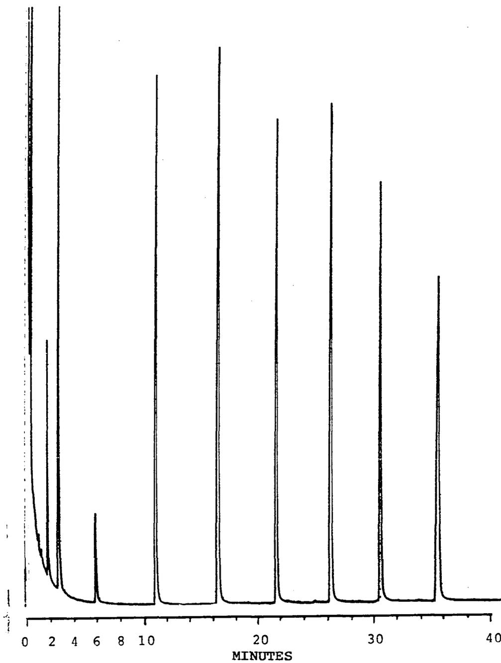
Figure 12. Gas chromatogram of n-alkanes C<sub>9</sub>-C<sub>18</sub> by trap-precolum capillary
