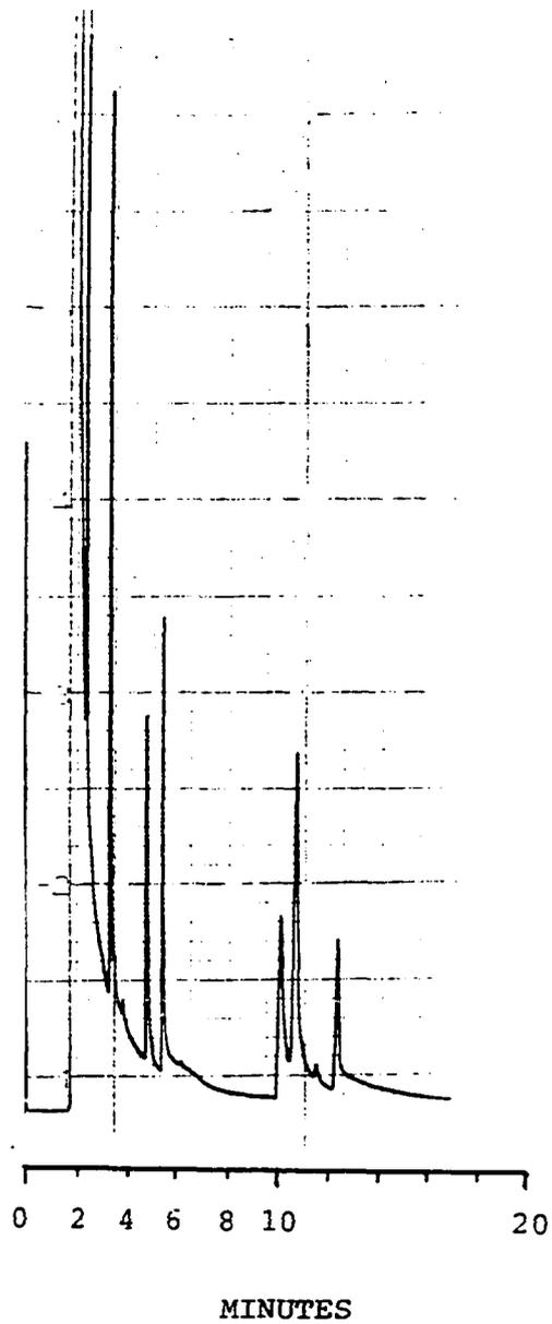
Figure 14. Gas chromatogram of C<sub>4</sub>-C<sub>9</sub> alcohols by trap-precolumn capillary SE-54, 30m, 80°C for 8 min, then 80°-160°C, 10°C/min.
