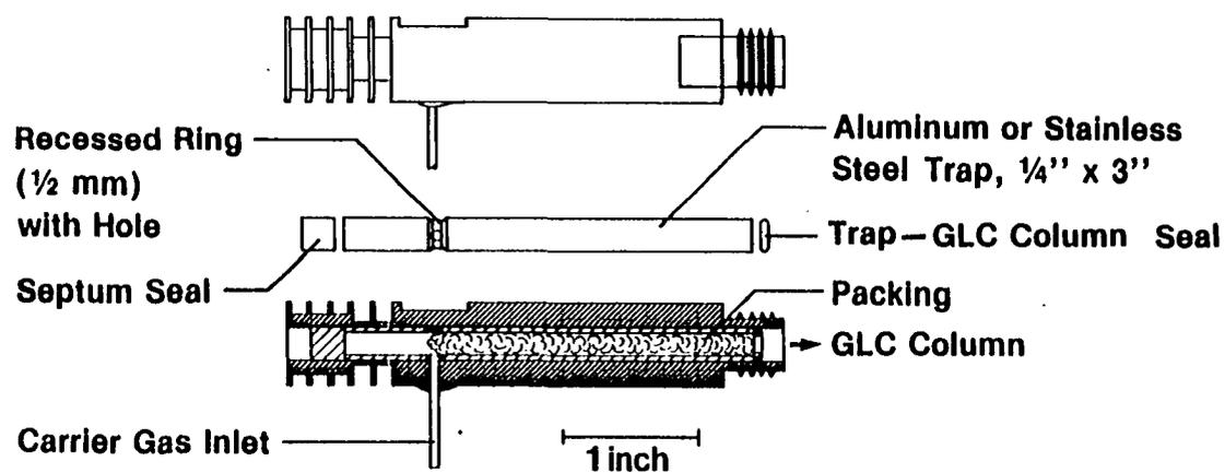
Figure 6. Modified gas chromatograph injector and resin trap assembly
