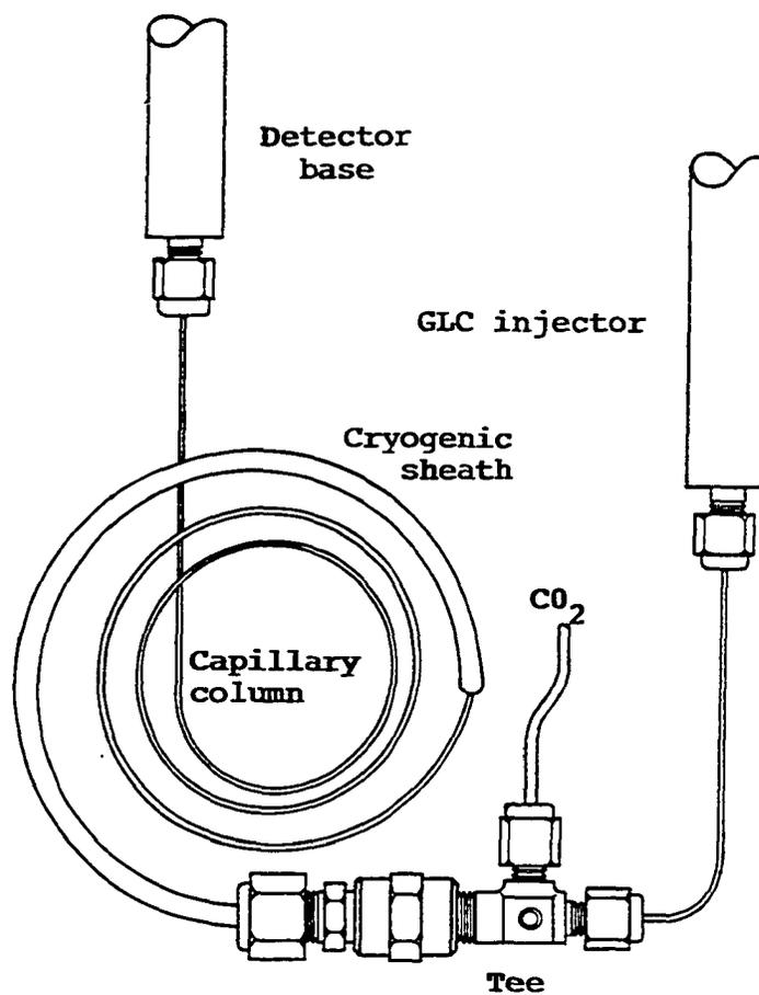
Figure 8. Cryogenic focus Mega-bore capillary GLC
