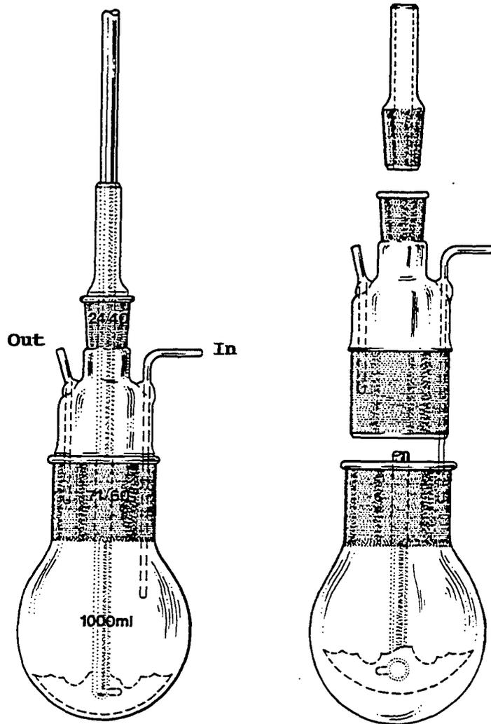
Figure 5. Closed cell model culture vessel, with sweep gas and stirring
