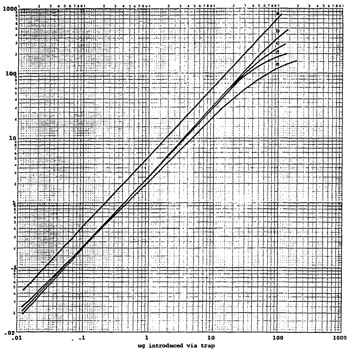
Figure 17. Standard curves of selected model volatile compounds by Tenax<sup>RT</sup> trap-GLC
