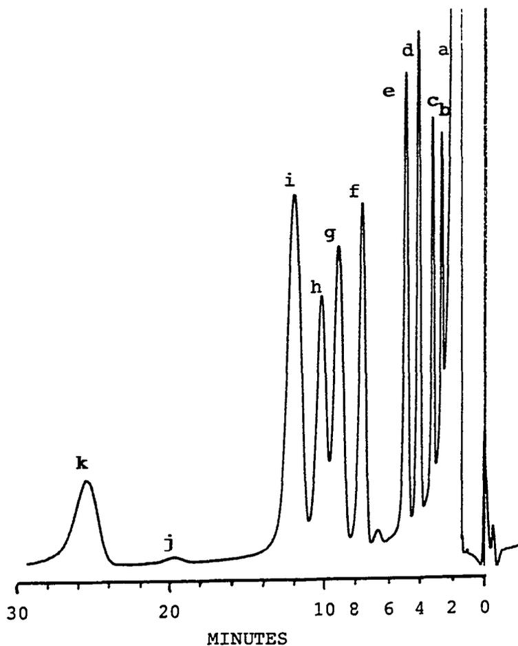
Figure 10. Gas chromatogram of a model volatile standard mixture in water
