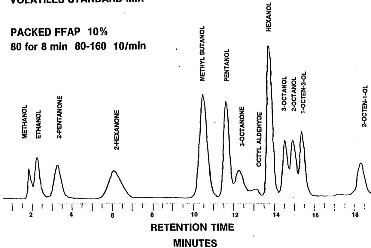
Figure 11. Gas chromatogram of a model volatile standard mixture in water, temperature programming 10% FFAP, 80°C for 8 min, then 80°C-160°C, 10°C/min., Finnigan 4500 GC/MS/DS
