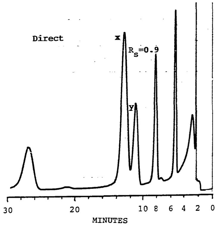
Figure 19. Comparison of resolution effects due to Tenax<sup>RT</sup> versus Tenax<sup>RM</sup>/carbon trap introduction to GLC
