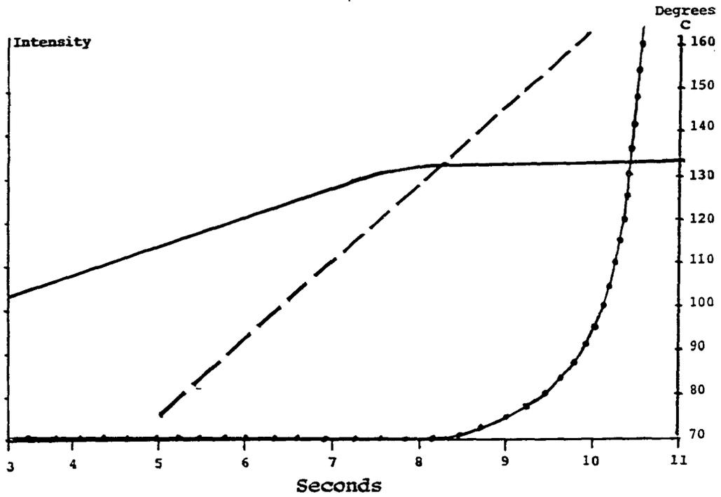
Figure 20. Heating cycle time effects on sample cup temperature, volatile standard recovery, and appearance of scorch products
